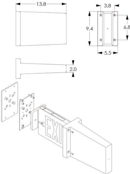
**APPLICATION/DESCRIPTION** Astralite has combined durability and style with dedicated mounting of this vandal and impact resistant Exit Sign. Gone are the days with the generic bubbles or oversized wire guards lagged to the walls. This product is designed to blend nicely in any environment without obstructive guards or cages. Use in gymnasiums, schools, and correctional facilities or anywhere rugged protection is required.
