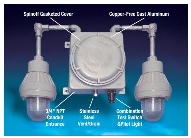
The **EXC Series** is completely self-contained and weather resistant, maintenance-free Nickel-Cadmium power system which provides safe emergency lighting in hazardous area locations. Cast copper-free aluminum housing; gasketed cover spins off for easy access to battery and electronics. A variety of fixtures and exits are available for mounting either directly to the housing or remotely which offers complete job flexibility.
