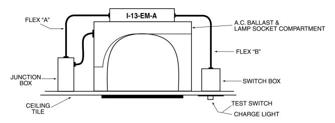
INSURE WIRING IS IN ACCORDANCE WITH THE NATIONAL ELECTRICAL CODE AND LOCAL REGULATIONS.
