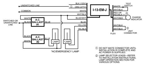
③ TEST ACCESSORY LEADS-REFER TO INSTALLATION INSTRUCTIONS FOR PROPER POLARITY WIRING.
