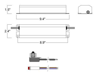
A test switch and charging indicator light is provided.
