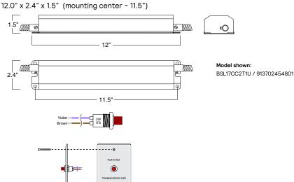
A Test/Monitor Plate with an illuminated test switch/charging indicator light is provided.
