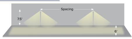
Multiple Unit Spacing (7.5' Mounting Height) Path Width Spacing CU2HL (2.7 Watt lamps) 55' 6' CU2HL (5.4 Watt lamps) 95' 6'
