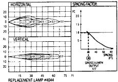
SPACING FACTOR Indicates the proper spacing between lamps to the chosen illuminance level (fc) ± 20%. ISOFOOTCANDLE CURVES Show distances in feet and isocurves in footcandles.
