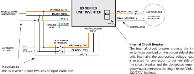
The IIS Inverter utilizes two sets of input leads: one to provide unswitched power to the inverter system and a second to serve as a normal power input to the lighting load. Any switch for the designated emergency circuit will be present on the Normal Power Input leads. For Emergency Operation Only applications, the Normal Input leads are not needed and would remain disconnected and capped.
