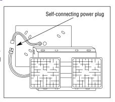
The ECS-2's battery lockout feature is an AC activated load switch that prevents the battery from discharging until the unit is energized with AC power. This allows the contractor to install the unit and connect the battery in one convenient operation.
