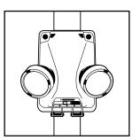
Vertical orientation for pole or column mounting.
