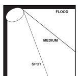
Field-adjusted beam pattern for composite lamps.
