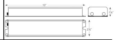
\* When battery packs are remote mounted, the remote distance cannot exceed 1/2 of the distance from ballast to lamp specified by the A.C. ballast manufacturer. The maximum allowable remote mounting distance is 50 feet.
