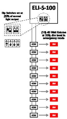
Note: dimming drivers are less efficient at reduced power. This inefficiency must be accounted for in the design.
