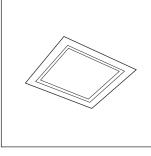
Fully-recessed mounting accessory kit – ELA FRK. (1/4" rough-in opening)
