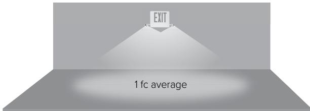
Meets Life Safety Code minimum illuminance of 0.1 fc and average illuminance of 1.0 fc. Assumes open space with no obstructions, mounting height of 7.5', ceiling height of 9' and reflectances of 80/50/20. Photometry files available on the Dual-Lite web site ([www.dual-lite.com](http://www.dual-lite.com)).
