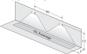
Using multiple LED-52 (4W) units mounted at a typical 7.5' height delivers 30' on-center spacing with a 6' wide path of egress.
