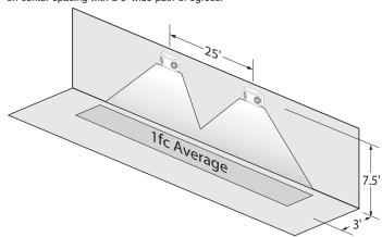
Using multiple LED-51 (2W) units mounted at a typical 7.5' height delivers 23' on-center spacing with a 6' wide path of egress
