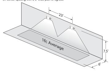
Using multiple LED-52 (4W) units mounted at a typical 7.5' height delivers 40' on-center spacing with a 3' wide path of egress.
