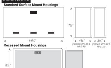
½" Extrusion from wall after installation
