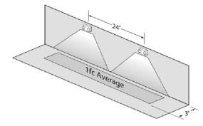
Using multiple units mounted at a typical 7.5' delivers 20' center-to-center spacing on a 6' wide egress path.
