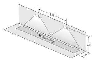
Using multiple NFT-HO units (5.4W lamps) mounted at a typical 7.5' height delivers 115' on-center spacing with a 6' wide path of egress.
