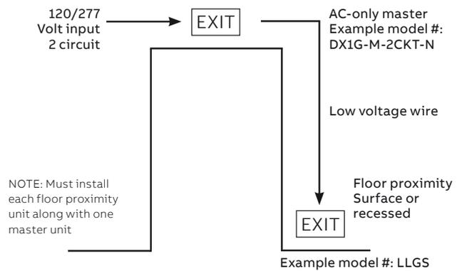
NOTE: Must install each floor proximity unit along with one master unit
