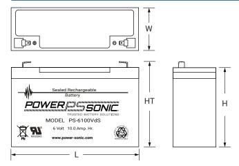
L: 5.94 (151) W: 2.00 (51) H: 3.70 (94) HT: 3.93 (100) Tolerances are +/- 0.04 in. (+/- 1mm) and +/- 0.08 in. (+/- 2mm) for height dimensions. All data subject to change without notice.
