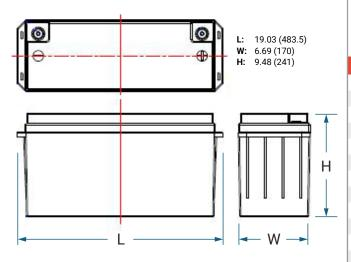
Tolerances are +/- 0.04 in. (+/- 1mm) and +/- 0.08 in. (+/- 2mm) for height dimensions. All data subject to change without notice.
