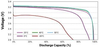
Charge: CC-CV 1C (max) 3.65V, 1250mA, cutt-off at 25°C Discharge: CC 1C, 2.0V cutt-off at different temperature
