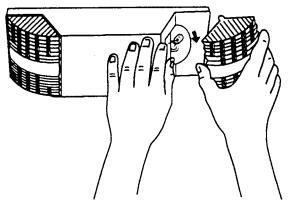
5. Change *light direction* by removing lens and adjusting socket position:
