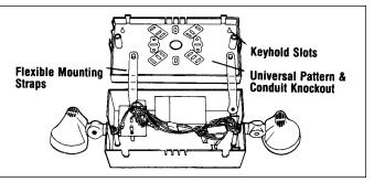
Installation is made easy by the two flexible hanger straps and the battery lockout feature.
