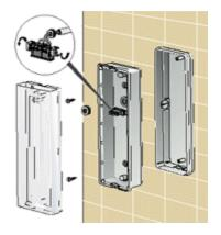
The housing and wiring can be installed and completed prior to the installation of the electronics. Finishing work can be completed without having to expose the STILE emergency lighting unit to possible damage or marking. Installation, cleanup and maintenance times are all reduced.
